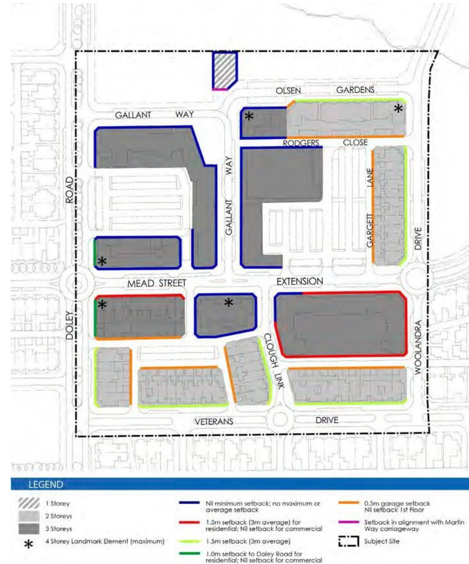
Figure 7: Building Heights and Setback Requirements
