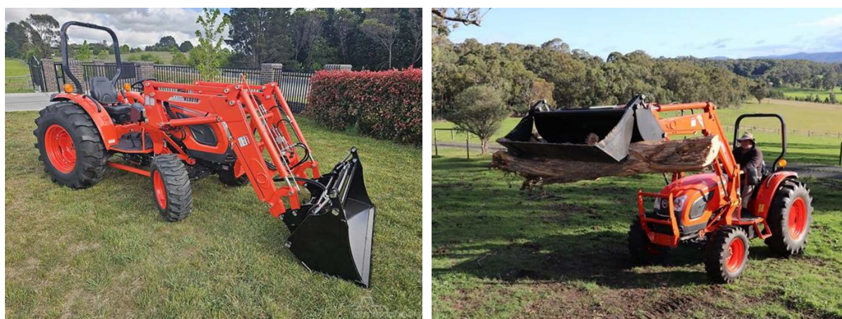
Figure 1: DK4810 with loader and 4-in-1 bucket (the proposed version will also have a canopy)
