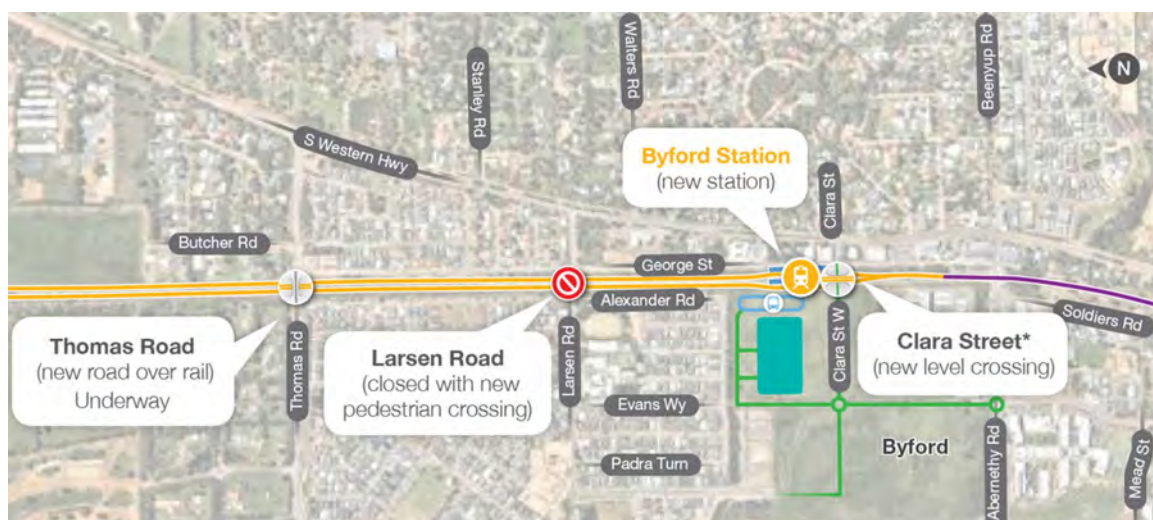
Figure 11: Location of the new Byford station and new railway crossing in the vicinity
