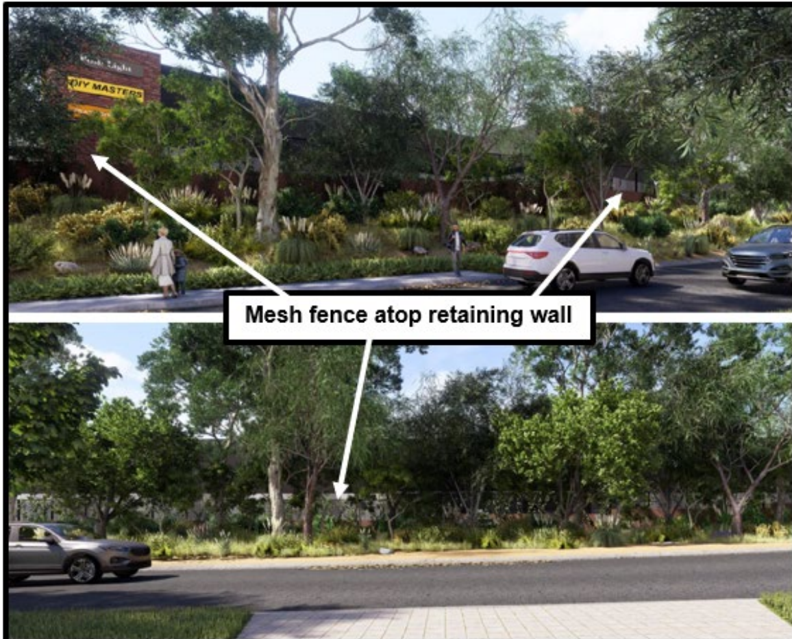
Figure 7: Chain link mesh fence atop retaining wall to south façade of the development
