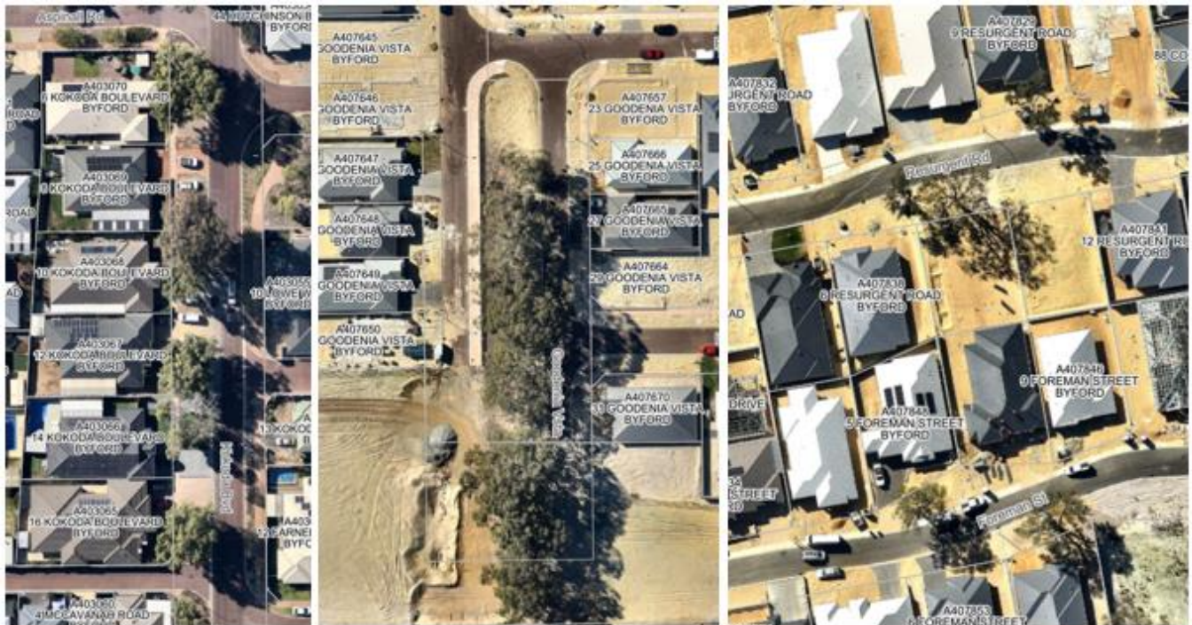
Figure 1 - Examples of successful tree retention. L-R: Kokoda Boulevard, Byford (wide verge); Goodenia Vista, Byford (wide median); Resurgent Road and Foreman Street, Byford (meandering road alignment)
