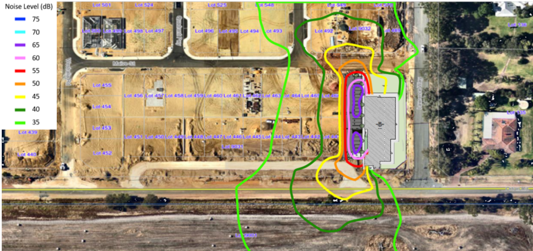
Figure 5: Night-time Environmental noise emission prediction ( L_{Amax} ) at 1.4 m above ground level (Assigned Level = 55 dB)
