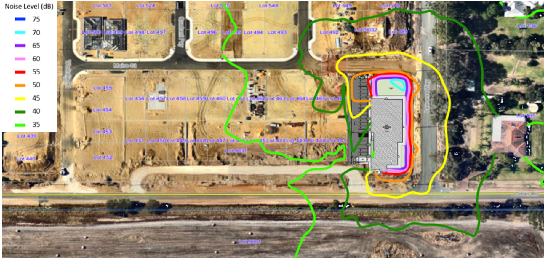
Figure 3: Daytime environmental noise emission prediction (LA10) at 1.4 m above ground level (Assigned Level = 45 dB)
